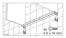
Screw the spacer strip to the bottom of the sides of the housing, flush with the rear wall.
